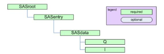
The minimum requirements for *reduced* small-angle scattering data. (<u>full image</u>) See <u>below</u> for the minimum required information for a NeXus data file written to the NXcanSAS specification.
